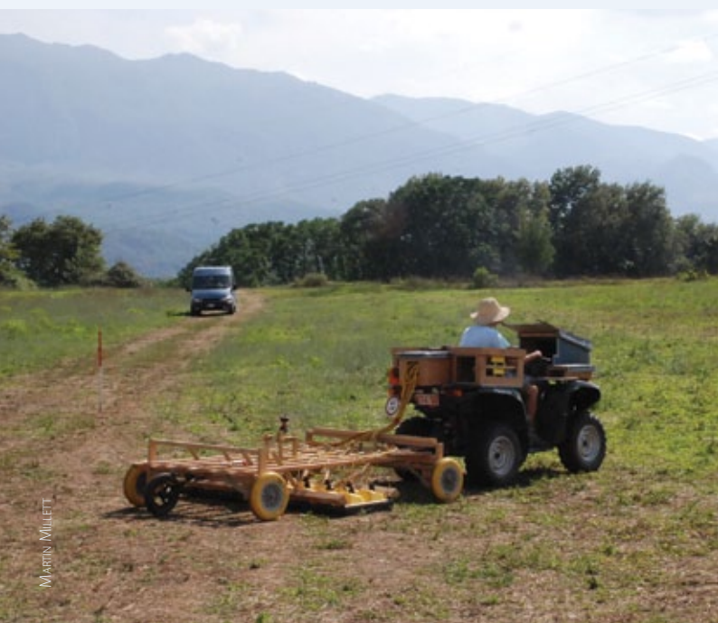
GPR survey in progress at Interamna Lirenas, Italy.
