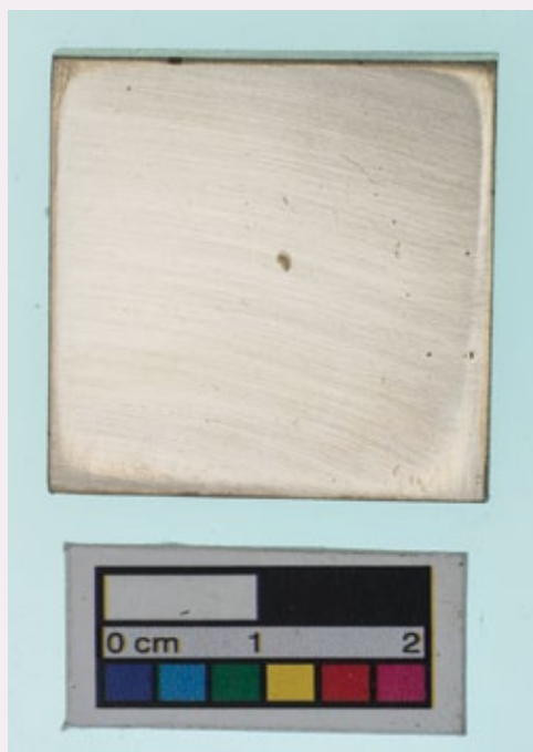
One of 70 experimentally produced metal pellets (Cu 80 per cent wt-Sn 20 per cent wt).
