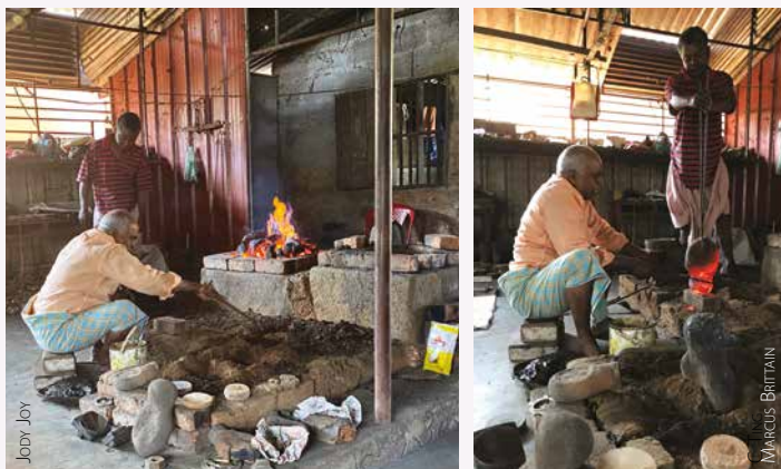
A master craftsman and assistant prepare to cast the mirrors in clay moulds.
