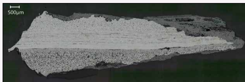
Metallography of the edge of a falcata sword from the Vetton necropolis of La Osera (Avila, Spain), revealing the composite construction of the blade, with different layers welded longitudinally; the lower, darker layer is medium-carbon steel, the middle area is pure iron and the upper layer is low-carbon steel. (Sample etched with 4% picral and 2% nital.)
