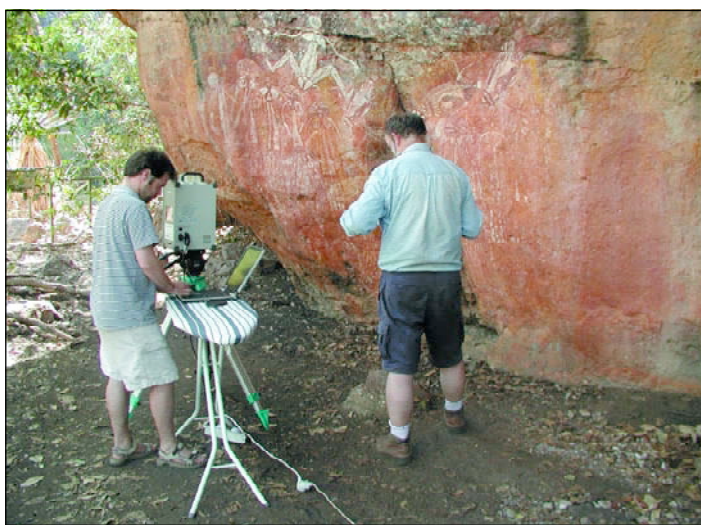
Jamie Hampson (2003–4 Cambridge MPhil student), left, uses a Minolta laser-scanner (kindly loaned to us by the Centre for Applied Research in Educational Technologies) to make a high-resolution three-dimensional record of the eroding surface at Anbangbang.
