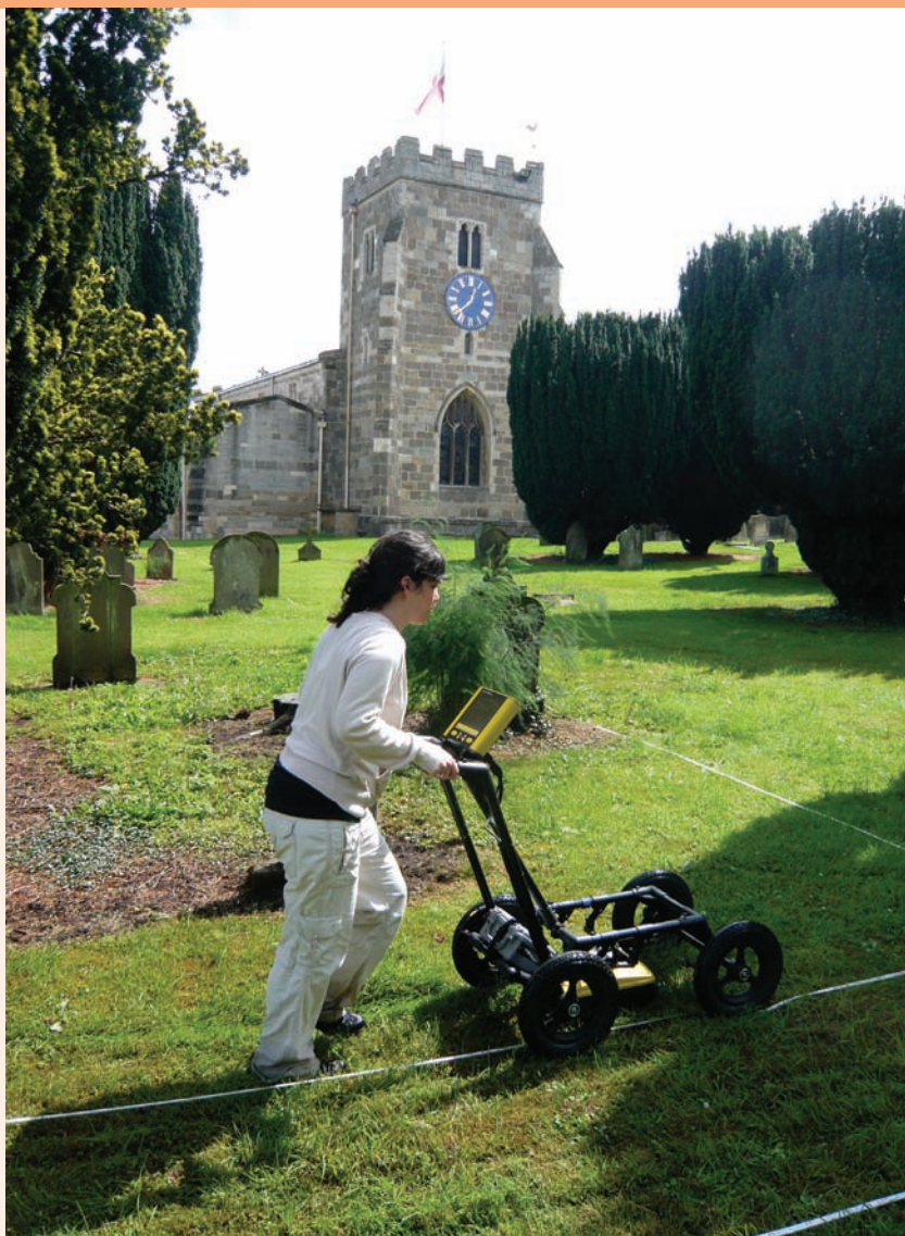
Ground Penetrating Radar survey work in progress at Aldborough.
